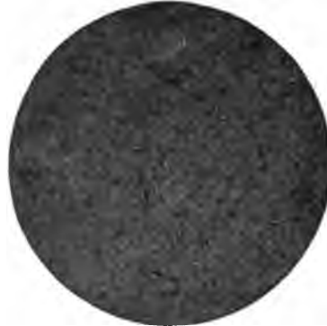
Fig. 18. Steel quenched at Correct Hardening Temperature
